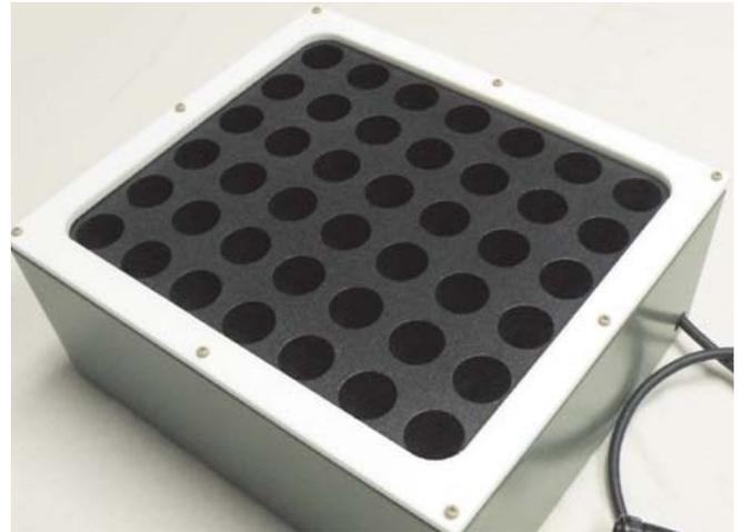
The QBlock Digester has 42 positions for 50ml vials. The graphite block is encapsulated in high efficiency insulation and enclosed in Teflon® coated exterior box which gives contamination free and repeatable digestions. It is engineered to be thermally secured from five sides allowing minimum heat dissipation. It is the only hot block in the market which reaches adequate temperature for tri-acid digestion.
