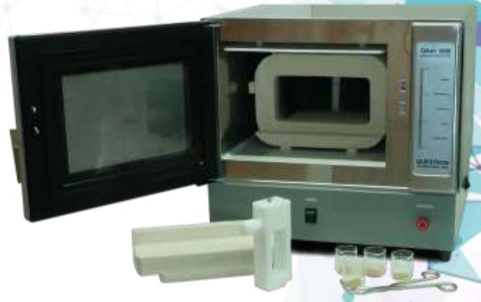
Microwave ashing is an innovative analytical sample preparation method that replaces the traditional ashing technique using a resistively heated muffle furnace. While maintaining the basic tried and tested principles of ashing, replacing the resistive heating with microwave heating offers distinct advantages, chief among them being speed, reduced energy cost, high sample throughput, reproducibility in results, cleaner working environment and increased operator safety.
